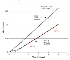
Figure 2: Rate curves of hematoxylin auto-oxidation in the absence and presence of CuZnSOD. SOD units as shown represent the concentration of enzyme added to the reaction mixture. The experiment was performed at room temperature (25°C) without a constant temperature cuvette holder.
