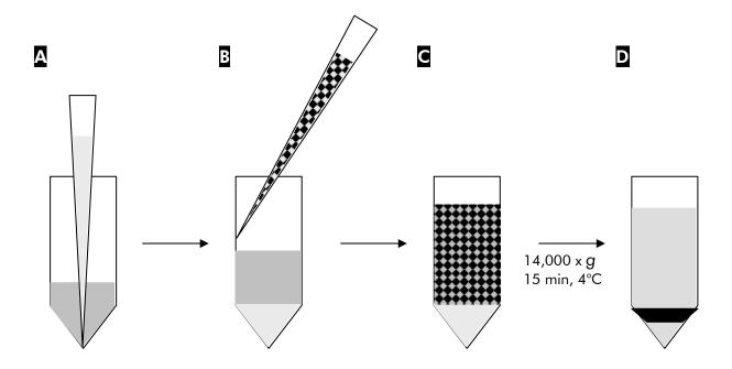
Figure 3  $\triangle$  In a 2 ml tube,  $500 \, \mu$ l Disruption Buffer is pipetted under  $750 \, \mu$ l Mitochondria Purification Buffer.  $\square$  — The crude mitochondria preparation from protocol step 10 is layered on top of the Mitochondria Purification Buffer.  $\square$  After centrifugation, mitochondria are concentrated in a band towards the bottom of the tube.
