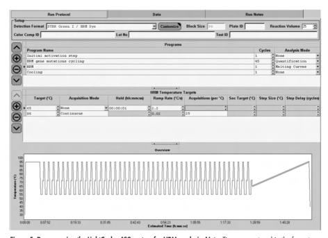
Figure 5. Programming the LightCycler 480 system for HRM analysis. Note: Times are entered in the format hh:mm:ss. Program the cycling protocol described in Figure 4. For HRM analysis, use 00:00:01 (1 s) at 65°C and 95°C. Select "Continuous" for "Acquisition Mode" with 25 acquisitions per second, resulting in a ramp rate of 0.02°C/s. Following HRM, samples should be cooled after the last cycle by entering 00:00:01 (1 s) at 40°C (not shown).
