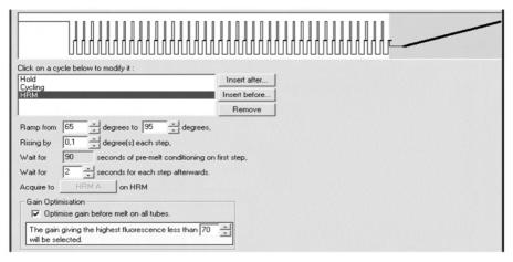
**Figure 2. Programming the Rotor-Gene system for HRM analysis.** Program the cycling protocol for gene mutation analysis described in Figure 1 and Table 2. For HRM analysis, ramp from 65°C to 95°C, rising by 0.1°C each step.
