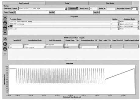
Figure 10. Programming the LightCycler 480 system for HRM analysis. Note: Times are entered in the format hh:mm:ss. Program the cycling protocol described in Figure 9. For HRM analysis, use 00:00:01 (1 s) at 65°C and 95°C. Select "Continuous" for "Acquisition Mode" with 25 acquisitions per second, resulting in a ramp rate of 0.02°C/s. Following HRM, samples should be cooled after the last cycle by entering 00:00:01 (1 s) at 40°C (not shown).
