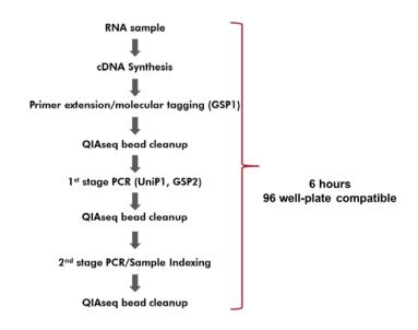
Figure 3. QIAseq Targeted RNA 2-stage PCR workflow.
