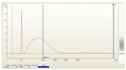
Figure 5. Local smear analysis: sample showing melanoma FFPE RNA. RNA from FFPE samples will be degraded; percentages will be returned based on the severity of degradation. In this sample, 30% of fragments are >200 nt.
