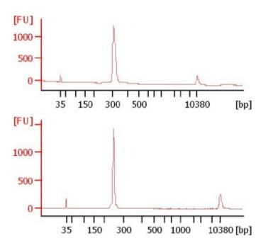
Figure 6. Bioanalyzer image of a QIAseq Targeted RNA Library prepared for sequencing on Illumina (above) or Ion Torrent (below) platforms. Peaks of approximately 300 bp or 250 bp are observed, respectively.
