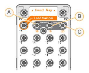
Figure 5. MiSeq reagent cartridge. A: position 18 for Read 1 Custom Primer; C: position 20 for Read 2 Custom Primer.
