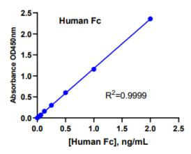
SUMMARY OF ASSAY PROCEDURE Add 100 µl of standard or sample to each well. Incubate at room temperature for 1 hours. Wash each well 4 times. Add 100 µl of 1× Detection antibody solution per well. Incubate at RT for 1 hour. Wash 5 times. Add 100 µl of TMB solution to each well. Incubate at room temperature for 20-30 minutes. Add 100 µl of Stop solution to each well. Measure absorbance of each well at 450 nm. Calculation
